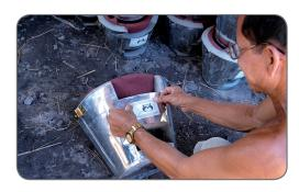
refractory liner also prevent heat loss. The metal sheet body cover provides further insulation and improves the durability of the stove. All these alterations serve to make the New Lao stove a more sustainable alternative to traditional cooking technologies.
