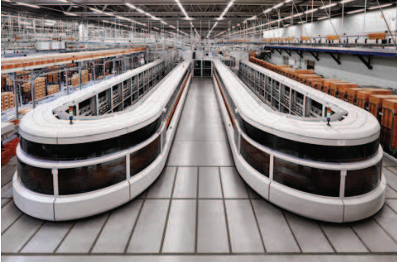
"Flatsorters" handle the fully automated sorting of mail shipments, and are able to process 38,000 items per hour
