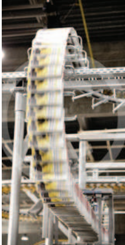
“Collators” enable the mechanical bundling of unaddressed direct mail items and is used in packing
