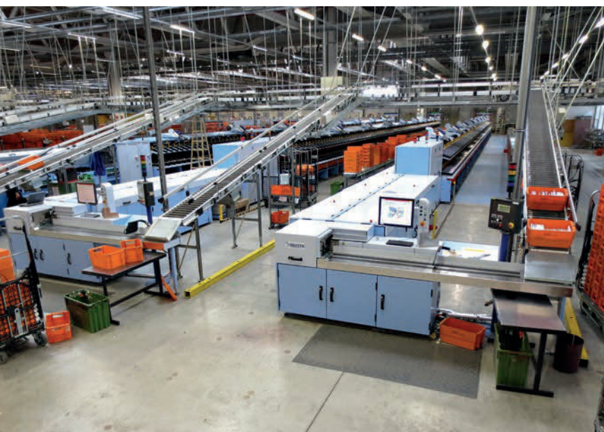
A modern letter mail sorting plant processes up to 46,000 letters per hour.
